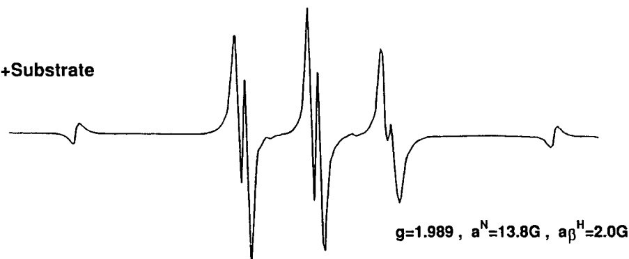
Figure 3. ESR spectra of phenyl- N -tert-butyl nitron-ketoprofen-derived radical adduct.
